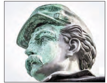
Bronze head of the Westfield Civil War Soldier monument has been partially cleaned with the Light Laser. The left side is light green and the right side is gray in color printings.
